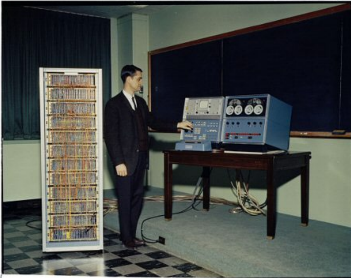
CP123-1.jpg, 03/27/1962, The LINC system demonstrated by its principal architect Wesley Clark at the Lincoln Laboratory Auditorium in March 1962.; LINC (Laboratory Instrument Computer), Approved for Public Release , LL History Book, Technology in Support of National Security, TiSoNS , TitNI
